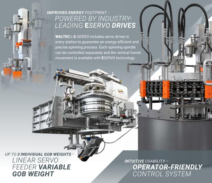
**WALTEC** supplies a wide range of feeders. The **E**SERVO feeder for variable gob weight allows producing different glass articles with various weights and designs easily. **WALTEC**'s linear **E**SERVO feeder offers multable speeds and excellent gob weight consistency for every distinct article.
