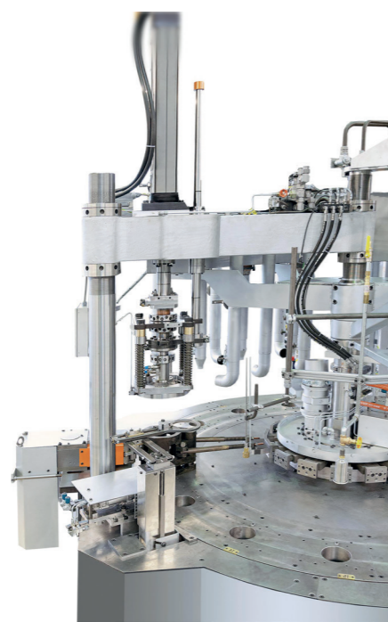
▶ Fig 1. The e-servo presses consume up to 85% less energy than the conventional method because they operate only when pressing force is needed.
